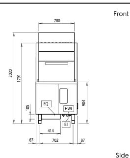
Drain Electrical inlet (power) FΩ **Electrical Outlet** HWI Hot water inlet Detergent connection Rinse aid connection
